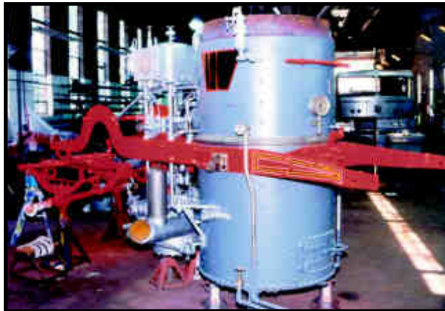
Ahrens steamer during refurb process in Fire Department shop.
